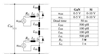
Fig. 25. The bridge leg comprising switches, stray inductances, gate drivers and (external) gate resistors. The values of the parameters are given on the right hand side for GaN and silicon switches. A sufficiently big DC link capacitor  $C_{\rm DC}$  is assumed and it is modelled with a constant voltage source. The parasitic inductance of the capacitor is neglected.
