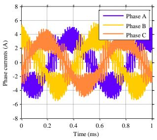
Fig. 19. Measured phase currents for 60 kHz PWM and the slotless machine at  $100 \ krpm$ . Input voltage of the inverter is  $122 \ V$ .
