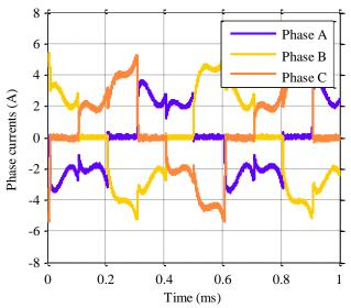
Fig. 18. Measured phase currents for PAM and the slotless machine at  $100 \ \mathrm{krpm}$ .
