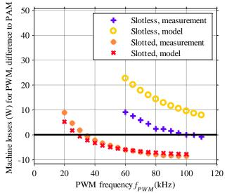
Fig. 22. Deviation of measured as well as modeled machine losses for both machines and a rotational speed of 100 krpm for PWM with respect to PAM.
