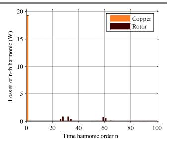
Fig. 11. Loss harmonic spectrum for PWM, a switching frequency of 50 kHz, the slotted machine and a rotational speed of 100 krpm.
