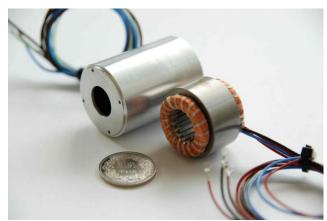
Fig. 7. Stators of the slotless (left) and the slotted (right) machines.
