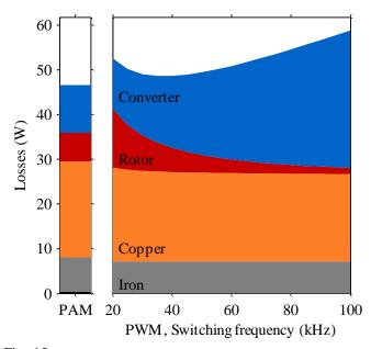
Fig. 15. Comparison of model results for the slotted machine and a rotational speed of 100 krpm. For PAM, the losses of the DC/DC buck converter whose efficiency is assumed constant at 98.5% are included in the converter losses.
