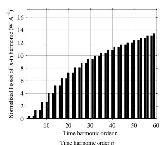
Fig. 8. Rotor losses caused by time harmonics for the slotless machine and a rotational speed of 100 krpm.
