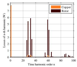
Fig. 12. Loss harmonic spectrum for PWM, a switching frequency of 50 kHz, the slotless machine and a rotational speed of 100 krpm.
