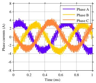
Fig. 21. Measured phase currents for 50 kHz PWM and the slotted machine at 100 krpm. Input voltage of the inverter is 130 V.
