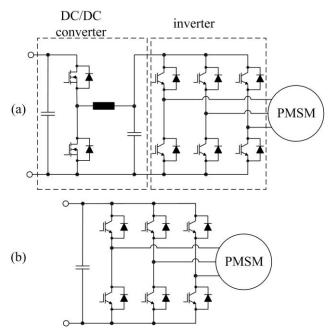
Fig. 2. The drive system comprising the power electronics converter and the machine. PAM converter comprising a DC/DC buck converter and a three phase inverter (a). Three phase PWM inverter (b).
