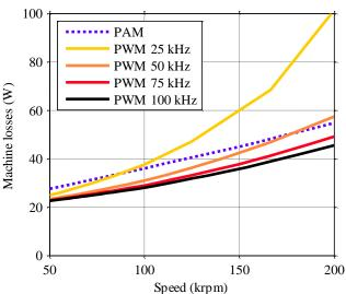
Fig. 16. Losses of the slotted machine over rotational speed.
