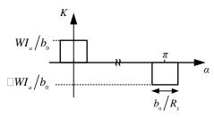
Fig. 5. The current sheet representation of a single coil built into two slots on opposite sides of the stator.
