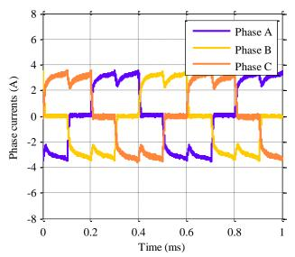
Fig. 20. Measured phase currents for PAM and the slotted machine at 100 krpm.
