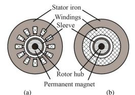
Fig. 1. Conceptual cross sections of typical slotted (a) and slotless (b) high-speed motors. The rotor hub does not exist in some machines.
