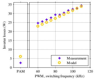
Fig. 23. Calculated and measured inverter losses for the slotless machine at  $100 \ \mathrm{krpm}$ .
