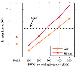
Fig. 26. Losses for PAM and PWM converters, both with GaN and silicon switches. The output power is 300 W. The DC/DC converter in PAM converter is switching at 100 kHz. For PWM, 12 W is the thermal limit for natural air cooling without heat sinks on the switches.
