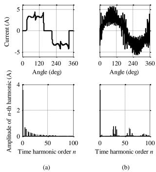
Fig. 3. Typical motor phase current waveforms and current harmonic spectra in the slotless machine for a rotational speed of 100 krpm, PAM modulation (a) and 50 kHz PWM modulation (b).
