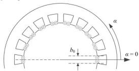
Fig. 4. Equivalent current sheet: current in a slot represented as a surface current density on the slot opening surface (circles).
