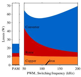
Fig. 13. Comparison of model results for the slotless machine and a rotational speed of 100 krpm. For PAM, the losses of the DC/DC buck converter whose efficiency is assumed constant at 98.5% are included in the converter losses.
