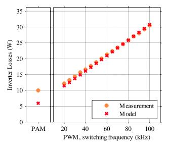
Fig. 24. Calculated and measured inverter losses for the slotted machine at 100 krpm.
