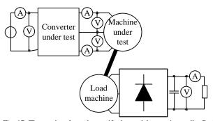
Fig. 17. The test bench used to verify the models experimentally. Both for PAM and PWM operation, the input power is measured at the inverter stage input (i.e., the losses of the DC/DC converter stage are not measured).
